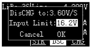
When selected as [Storage], it will prompt the target voltage to charge and discharge the battery. If the discharge mode is to recycle the discharge, it is also necessary to set the cutoff voltage of the battery. As shown below
