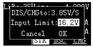
The high limit voltage of recovered. The default is 0.5V higher than the input voltage. Please set according to the maximum limit voltage of the input power supply. To cancel the operation, move the cursor [Cancel] or press [Exit]. Move the cursor to [OK], short press [OK] to start charging, and display the charging and discharging work interface.
