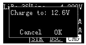
When selected as [Discharge], it will prompt the target voltage to put the battery. If the discharge mode is to recycle the discharge, it is also necessary to set the cutoff voltage of the power battery. As shown below
